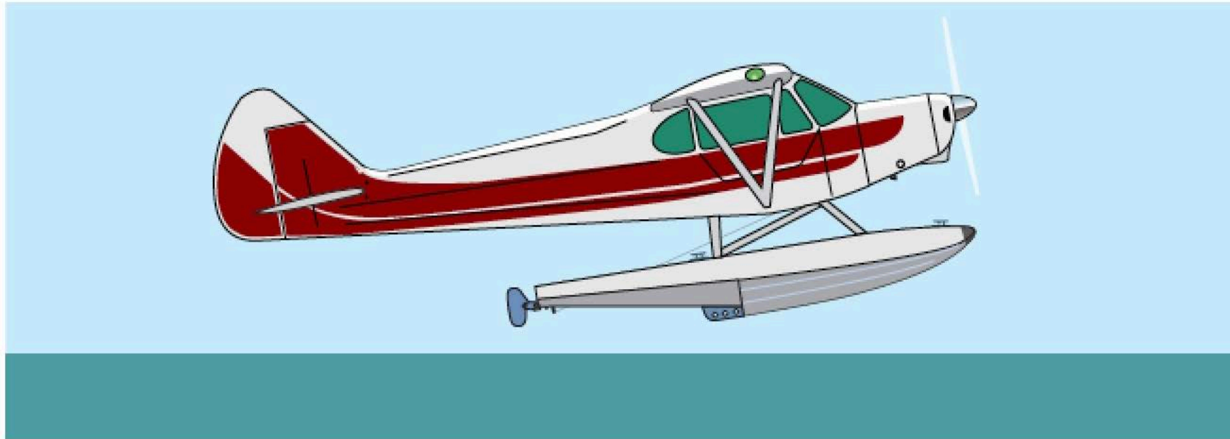
Figure 6-2. The touchdown attitude for most seaplanes is almost the same as for taxiing on the step.
